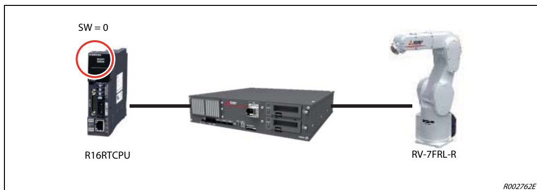
Fig. 5-7: Connect the robot to the controller CR800-R
