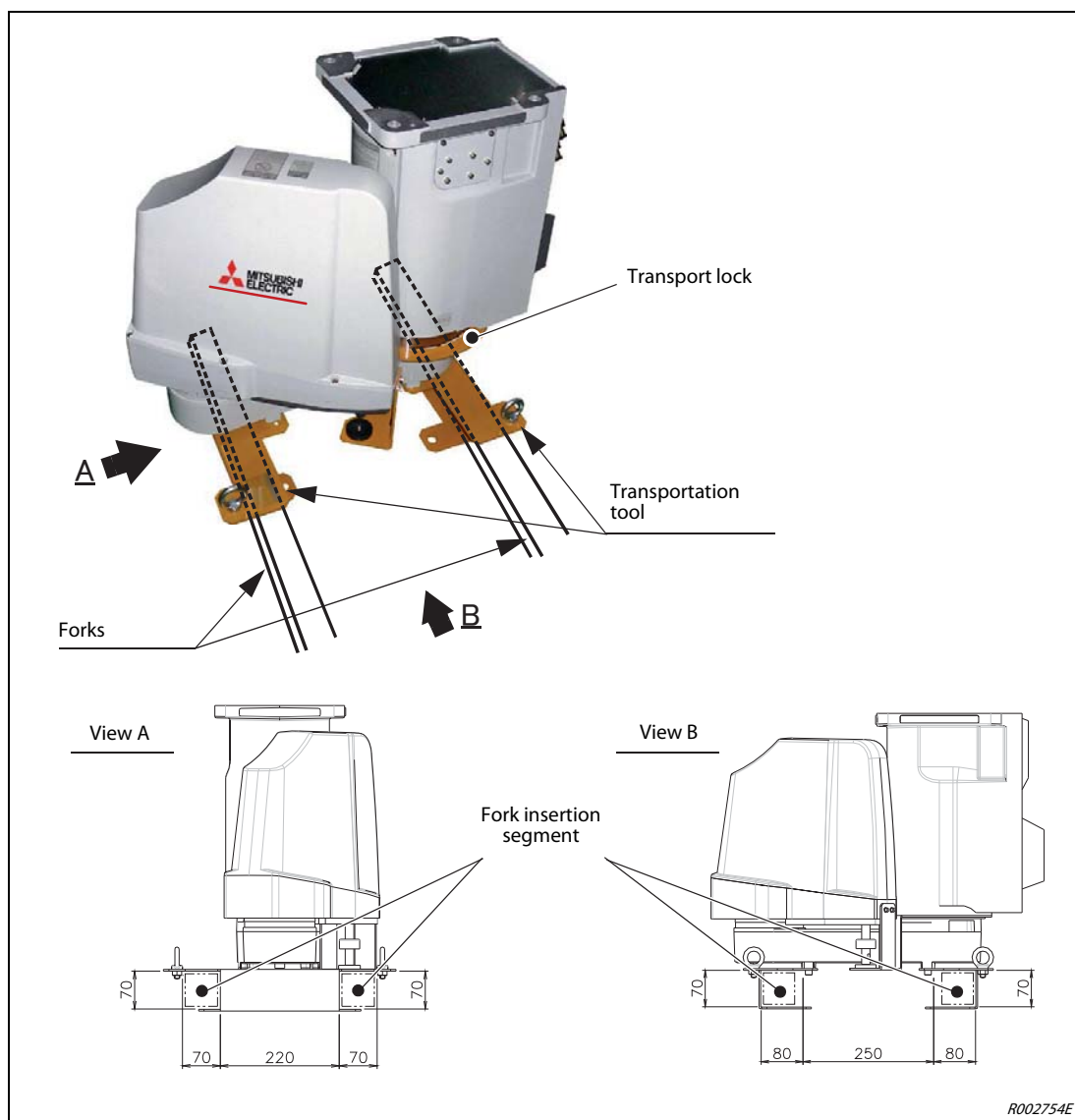
Fig. 3-10: Fork insertion segment of the robot
