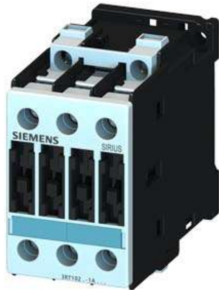
CONTACTOR, AC-3 4KW/400V, AC 24 V, 50/60 HZ, 3-POLE, SIZE S0, SCREW CONNECTION
